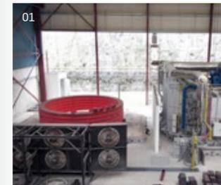
Manufacturing process\_ Once the forging process has been completed the flange is transferred to the turning center to remove the excess material from the raw flange to final size. Later, the drilling center drills the fixing points to join the modules of the tower.
