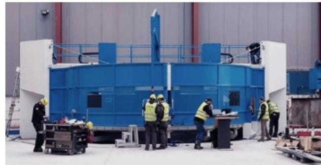
IBARMIA and GRI technicians during the final touches to the turning center prior to commissioning tests of the machine.
