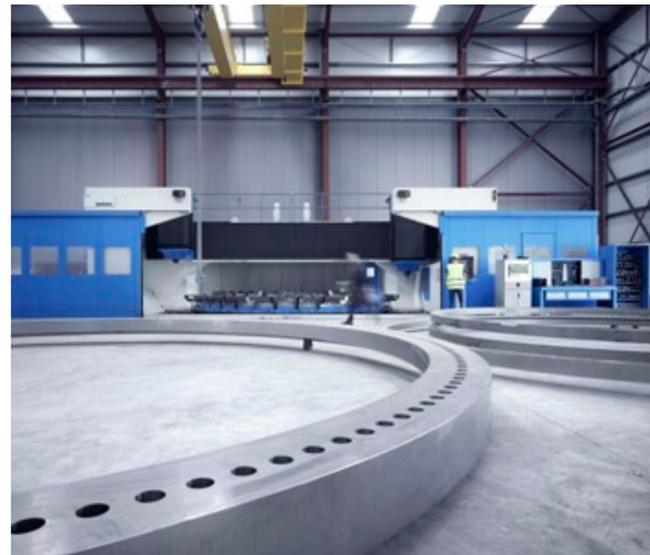
In 2005, IBARMIA developed a new concept of high-productivity drilling centre that revolutionized the market for drilling large flanges. It arose from an order for a machine with gantry architecture and one of its main requirements was that it had to be as strong as a tank because at IRAETA they frequently "destroyed" their machine tools by constant use.
