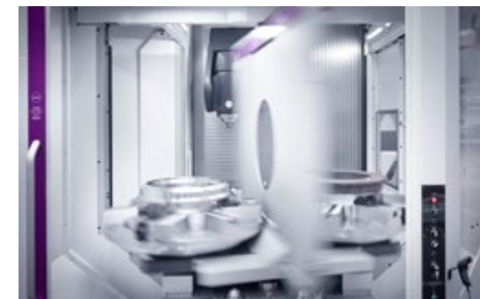
Rotopallet APC system for T12 & T16 A rotary double fork device on the frontside of the machine makes a quick change of two pallets.
