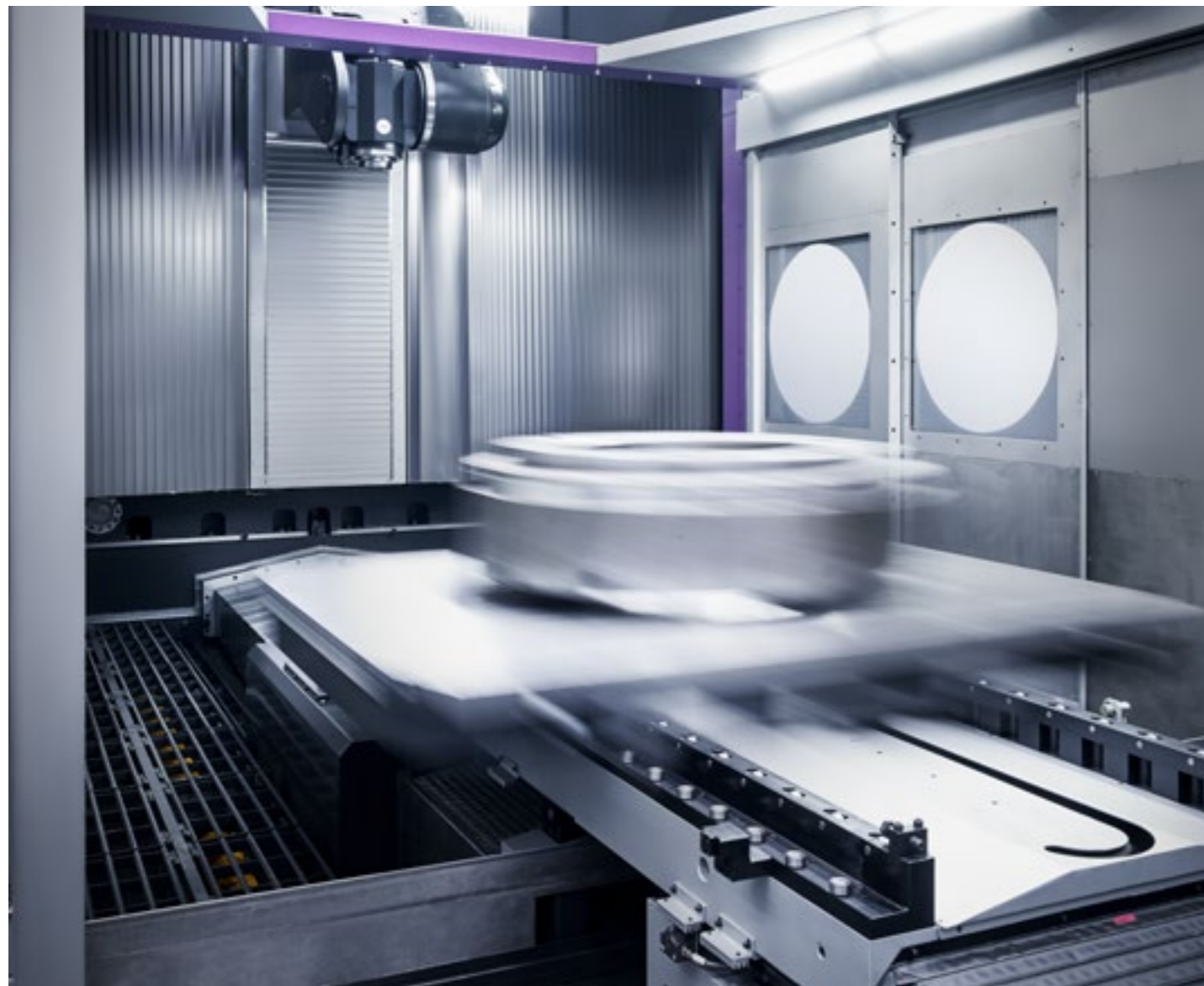
In the picture above, pallet changing on a THR 36 machine. These flexible manufacturing systems respond to large series and single unit fabrication, making them attractive to companies and sector of every size. (View on pages 40-41).
