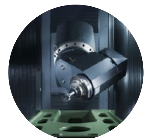
THC UNIVERSAL HEADSTOCK B axis system. Strokes: 180° +/-15°
