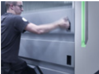
Loading of extra long parts through the side panelling which is easily removable. (Standard).
