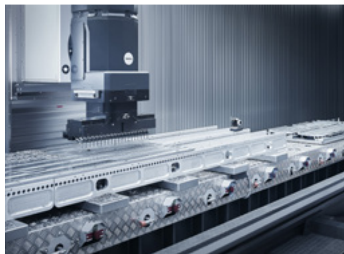
Customize the fixed table with hydraulic connections for automatic clamping devices.
