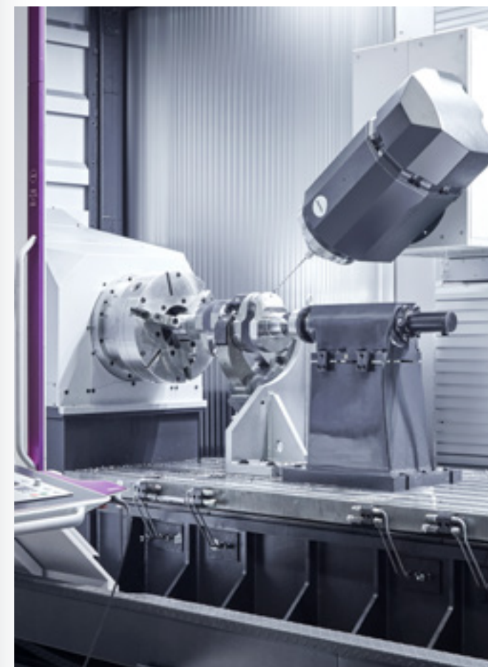
Complete the fixed table configuration by integrating a wide range of devices as steady rests, tailstocks, bolt-on rotary tables or supports...
