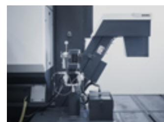
Chip conveyor with integrated coolant tank.
