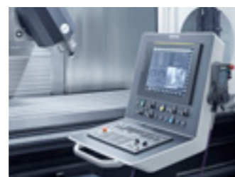
Fanuc 31i-B control with 19" touch screen. (Vertical screen in STAR 1500).
