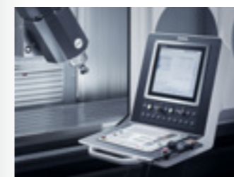
Heidenhain TNC 640 HSCI control.
