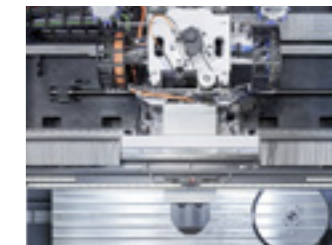
Linear axes are verified by laser interferometers according to VDI/DGQ3441 and circularity accuracy by ball-bar.
