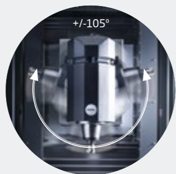
ZVH SPINDLE HEAD B axis, 4th movement. Continuous tilting head / Torque motor. +/-105°
