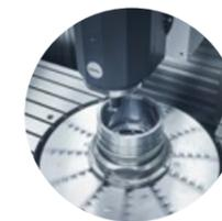
C axis integrated rotary tables for vertical 5 axis milling and turning operations.
