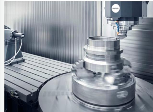
**ADD VERTICAL TURNING CAPACITY** \_ Into these integrated C axis rotary tables. **C axis turning & milling rotary tables** up to  $\varnothing 1200$  mm / 6000 kg / 500 rpm / 83 kW / 4000 Nm.
