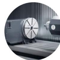
A-C axis bolt-on rotary tables for machining up to 5 axis / 5 faces.
