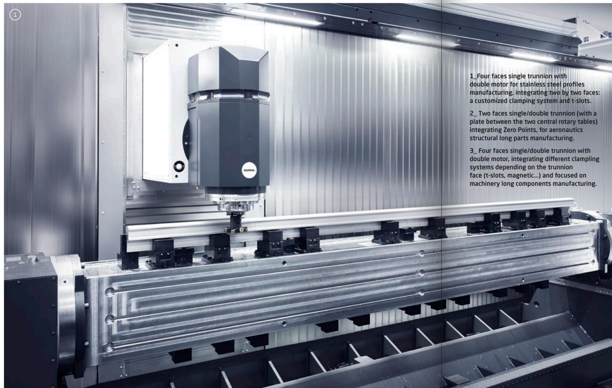
1\_ Four faces single trunnion with double motor for stainless steel profiles manufacturing, integrating two by two faces: a customized clamping system and t-slots.
