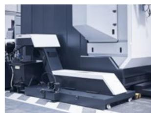
Chip conveyor with integrated coolant tank. (Standard).
