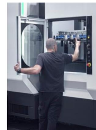
Chain system or polar type ATC magazines available, in both cases located at the right side of the machine for a easy load / upload tools while the machine is running.
