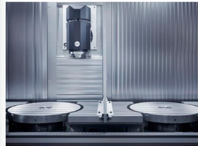
**C AXIS INTEGRATED ROTARY TABLES** \_ milling rotary tables fully covering the Y axis for 5 axis / 5 faces machining operations. Up to 25 rpm /  $\varnothing 1500$  mm swing / 3500 kg. Combine these rotary tables according to your machining requirements.
