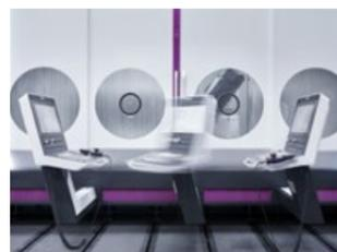
Moving and light control panel with 360° rotation over the entire longitudinal travel. (Standard).
