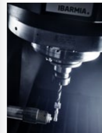
MACHINE PRESETTING DEVICES The program offers the possibility of add a wide range of tool measuring and touch systems integrated in the machine.
