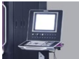
Moving control panel with 19" touch screen.
