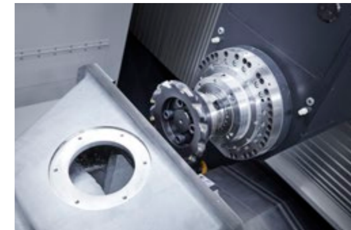
A WIDE RANGE OF ELECTROSPINDLES AVAILABLE The program offers a large variety of spindles available, to cover from high dynamics machinings to works on the hardest materials by high torque spindles.
