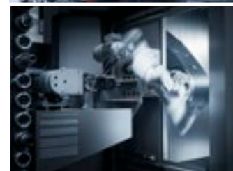
120-240-360 positions chain driven tool magazine with servomotors.
