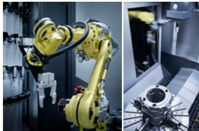
LARGE CAPACITY POLAR TOOL MAGAZINES Managed by arm robot, combining tool changing with special tools and heads changing.
