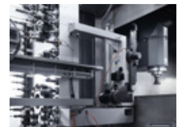
60 positions chain driven tool magazine with servomotors.
