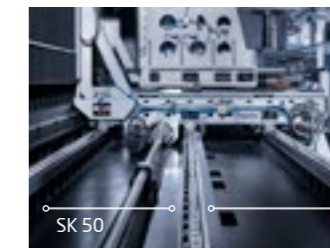
#50 Electrospindle Power in S1 (100%); S6 (40%) 74 kW / 84 kW Total available power from 4000 rpm Torque in S1 (100%); S6 (40%) 300 Nm / 452 Nm Maximal rotation speed 12.000 rpm
