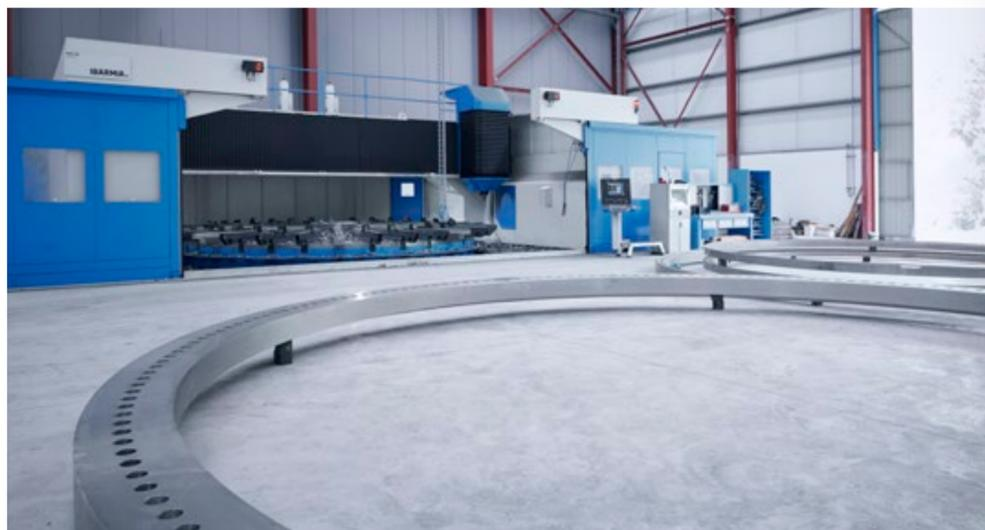
TODAY, THE NEW MACHINING LINE IS PRODUCING PROBABLY THE LARGEST FLANGES TO BE FOUND ON THE WIND TURBINE SUPPORT STRUCTURE MARKET.
