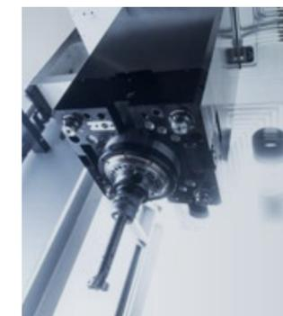
**Live Spindles** integrated inside the RAMs are a key element, both as the direct solution to vertical milling, drilling, threading or boring operations and transmission element to drilling and grinding interchangeable heads.
