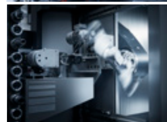
120-240-360 positions chain driven tool magazine with servomotors.
