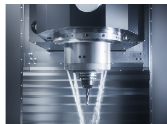
External coolant system around the spindle.
