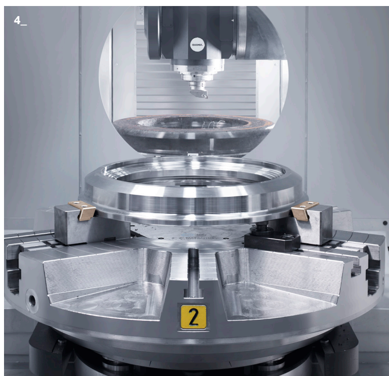
4_ THR 12 MULTIPROCESS equipped with Rotopallet for the maintenance of metro-train wheels. Top of the range among models with pallet changing (see page 19), this system increases the production and autonomy of the machine while minimising its occupation in plant.
